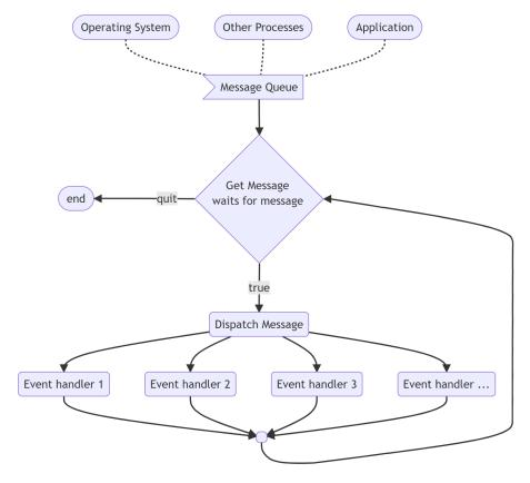
The basic mechanics of an *event loop*, regardless of the platform, are the following:
