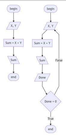
If we compare both program flow diagrams, the difference becomes more obvious. The first program has a plain, linear flow, and the second one has a distinct *main loop* logic implemented.
