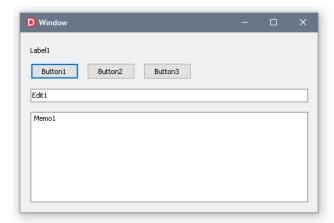
One window is pretty obvious in the above image... but, it is not the only one. Every button is a window, the edit is a window, the memo is a window. No, I didn't forget about the label, the label is not a window. And there are also invisible windows not meant to display anything.
