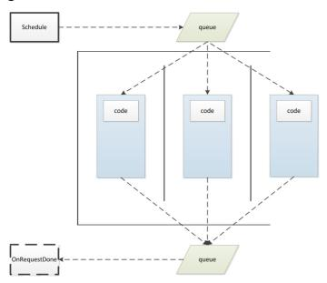
When you call Parallel. BackgroundWorker. Execute, OmniThreadLibrary starts your task in one or more threads. Task code is wrapped in a wrapper which receives requests from the owner, calls the task to process request and returns result to the owner.
