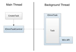
The task has access to the IOmniTask interface and can use it to communicate with the owner (the part of the program that started the task). Both interfaces are explained in full detail in chapter Low-level multithreading.
