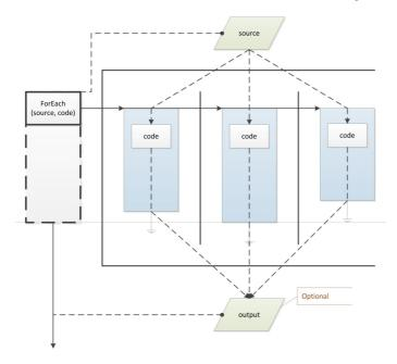
When you use Parallel. For Each, OmniThreadLibrary starts multiple background tasks and connects them to the source through a serialization mechanism. Output is optionally sorted in the order of the input. By default, For Each waits for all background threads to complete before the control is returned to the caller.
