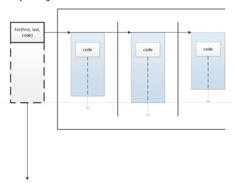
Parallel. For provides a simple way to parallelize a for loop. When you use Parallel. For, OmniThreadLibrary starts multiple background tasks, each working on a subset of for loop ranges. By default, For waits for all background threads to complete before the control is returned to the caller.
