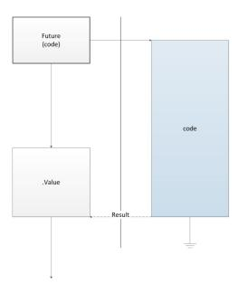
When you call Parallel. Future, a background task is started immediately. The task continues with its (possibly long) execution and the main thread can do some other work. When you need the result of the background calculation, call the . Value method, which will return the result immediately if it is ready or which will wait for the background code to complete its work if necessary.
