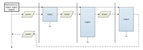
When you call Parallel. Pipeline, background tasks for all stages are started each in its own thread. The system also creates input queue, output queue and interconnecting queues.
