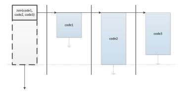
When you use Parallel.Join, background tasks are started in background threads. By default, Join waits for all background threads to complete before the control is returned to the caller.
