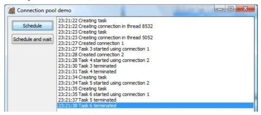
For the third demo, I restarted the app and clicked the Shedule button three times. Only two worker threads were created and two connections established and two tasks started execution. The third task entered the thread pool queue and waited for the first task to terminate, after which it was immediately scheduled.
