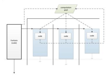
Parallel.ForkJoin creates a computation pool into which you can submit requests (subtasks). Each subtask can create multiple sub-subtasks which are again submitted into the computation pool.
