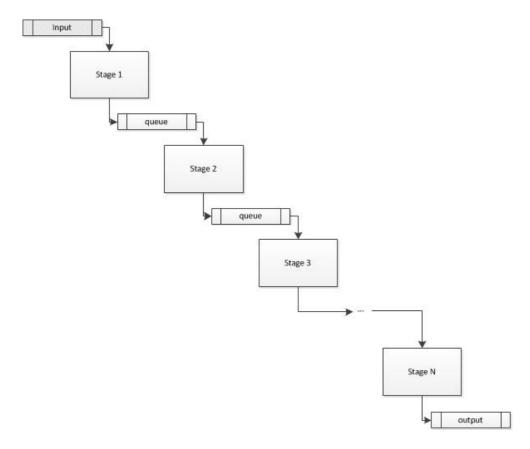
What is important here is that no stage shares state with any other stage. The only interaction between stages is done with the data passed through the intermediary queues. The quantity of data, however, doesn't have to be constant. It is entirely possible for a stage to generate more or less data than it received on the input queue.
