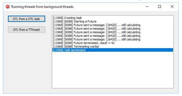
We can see that Future messages were generated in thread 18420, then passed through the parent thread 6088 and ended in the main thread 11968.
