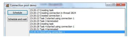
Now a new task was created (with ID 4), was scheduled for execution in the same thread as the previous task and reused the connection that was created when the first task was scheduled. There is no 5 second wait, just the 3 second wait implemented in the task worker procedure.
