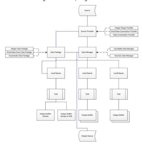
OtlDataManager unit contains four different source providers - one for each type of source that can be passed to the ForEach method. If there is a need to extend ForEach with a new enumeration source, I would only have to add few simple methods to the OtlParallel unit and write a new source provider.
