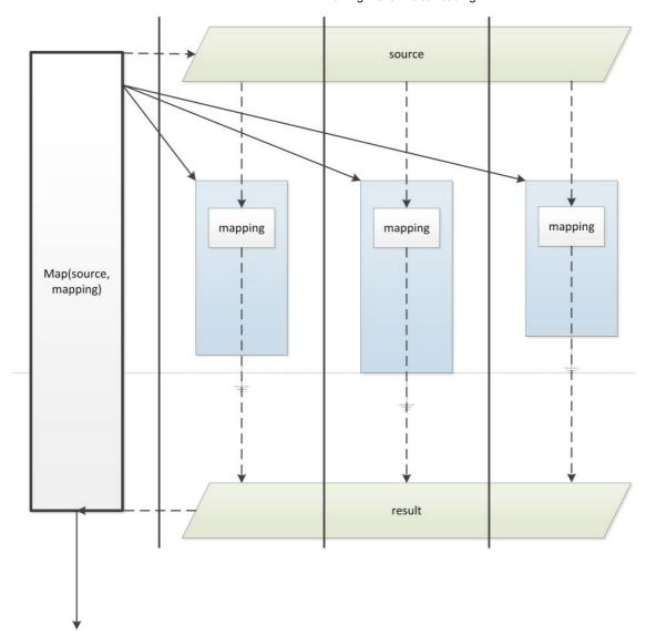
When you call Parallel. Map, a same background task is started in multiplie blackground threads (indicated by the bold vertical line). In each thread, this task runs some filtering function (provided by the programmer) on some subset of the input array and creates output array containing data returned from the filtering function. At the end, all output arrays from background workers are combined together into the final result.
