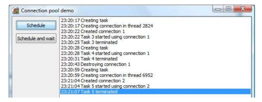
Let' s try something else. I was running the demo on my laptop with a dual core CPU, which caused the thread pool to limit maximum number of currently executing threads to two. By default, thread pool uses as much threads as there are cores in the system, but again you can override the value. (In releases up to [3.03], you could use at most 60 currently executing threads. Starting from release [3.04], this number is only limited by the system resources.)
