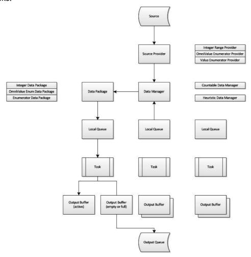
All this was designed to provide fast data access (blocking is limited to the source provider, all other interactions are lock-free), good workload distribution (when a task runs out of work before other tasks, it will steal some work from other tasks) and output ordering (when required).
