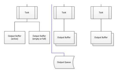
When we look at data reading/writing from perspective of one task, everything is very simple. The task is reading data from a local queue (which reads data from a data package, associated with some position) and writing it to an output buffer (associated with the same position).
