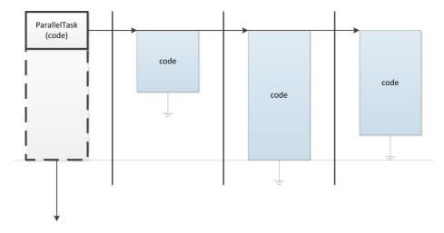
When you use Parallel.ParallelTask, same background task is started in multiple background threads. By default, ParallelTask waits for all background threads to complete before the control is returned to the caller.
