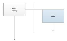
When you call Parallel. Async, code is started in a new thread (indicated by the bold vertical line) and both main and background threads continue execution. At some time, background task completes execution and disappears.
